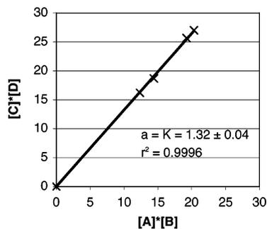
**Figure 1.** Calculation of the equilibrium constant for the reaction represented in Scheme 1 using a correlation between the concentrations of species  $[C] \times [D]$  and that of species  $[A] \times [B]$ .
